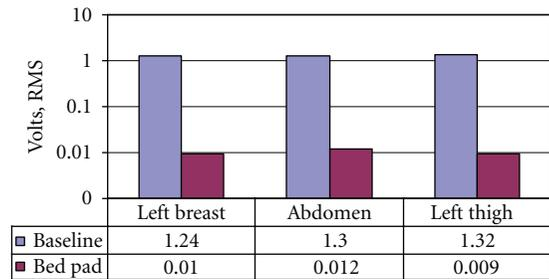
FIGURE 2: Effect of bed pad grounding on 60 Hz mode.
